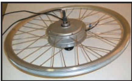
Photo 2 —This is the Crystalyte 408 brushless DC motor. The motor was ordered with the wheel and spokes already mounted. The axle was modified using a rotary tool in order to mount the four strain gauges.
