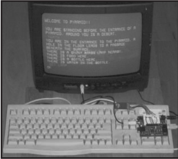
Photo 2 —I translated the classic Pyramid 2000 game into CCL, where it lives again on my Propeller demo board.
