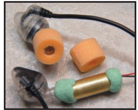
Photo 2 —A 7 x 22 mm brass tube resembles an ear canal closely enough to measure my Shure E2C earphone response. The foam plugs seal tightly in a real ear canal to exclude sounds that don't come from the electronics.
