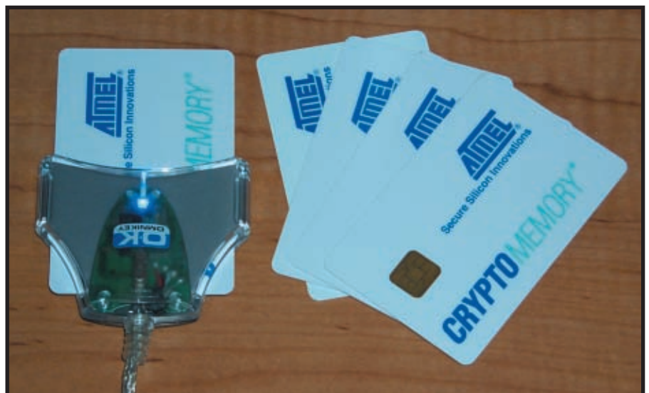
Photo 2 —Pick a card, any card. The AT88SC demonstration kit (AT88SC25616C-DK) packages the memory chips in Smartcard format and comes with a USB-based reader for connecting to your PC.
