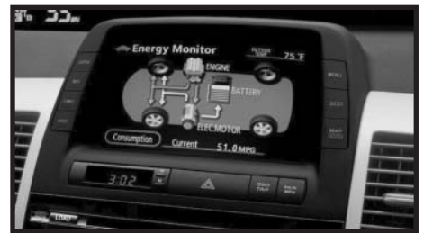
Photo 1—The Toyota Prius hybrid features a GUI that brings all vehicle functions to a central location on the dashboard. The real-time display of energy consumption and the dynamic interplay between internal combustion and the electric motor is fascinatingly educational.
