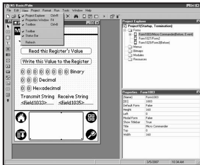
Photo 2 —The NS Basic IDE is similar to many development tools used in the Windows environment. From here you can design screens, write code, compile, and download to either hot-sync the application to your handheld or download into the Palm OS Emulator (POSE).
