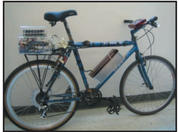
Photo 1 —This is our electronic bike. The ultracapacitor bank is mounted in a plexiglass case. The metal case in the middle of the bike holds the lithium-ion batteries. The red case on the handlebar holds the LCD and control buttons.
