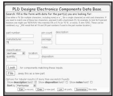
Photo 1 —This screenshot shows the start-up condition with one input field filled in. A search for all components manufactured by Texas Instruments will be started when the Look button is clicked. Options near the bottom of the window determine what happens if multiple part numbers are returned. In this case, the list will be sorted in part number order, and of the optional fields, only the “description” field will be displayed.
