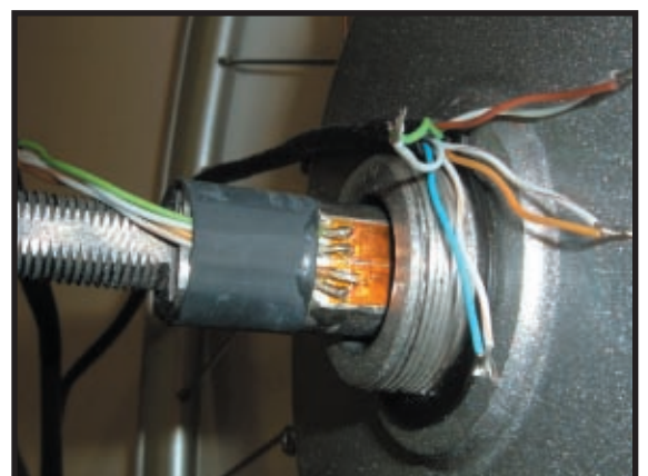
Photo 4 —The four strain gauges were mounted on the rear axle. The axle was ground flat to allow more deflection and make it easier to mount the strain gauges.
