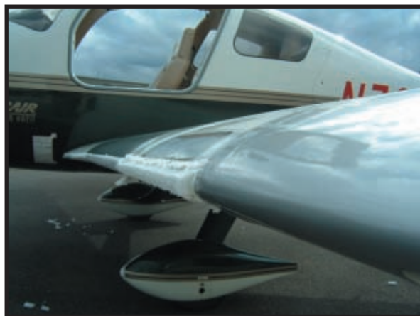
Photo 1 —The protected area covered by the gray heater is clean, while the unprotected landing light lens shows the severity of the icing where the test flight took place. (Popsicles fly poorly!) Also note the "nose caps" of ice on the wheel fairings, and the chunks of ice that are falling on the ramp as the unprotected areas of the airframe warm up after landing.
